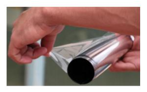
**Step 3 - Precut film:** Precut film to window size, leaving 2cm overlapping edge all around: prepare the film straight from the box, cutting from the hardcoat side with an sharp blade. Make sure the film is rolled with release liner outside (SR coating inside).
