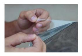
**Step 6a** - Using two pieces of adhesive tape, separate the release liner from the film.
