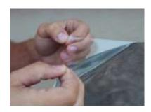
**Step 4:** Using two pieces of adhesive tape, separate the release liner from the film.
