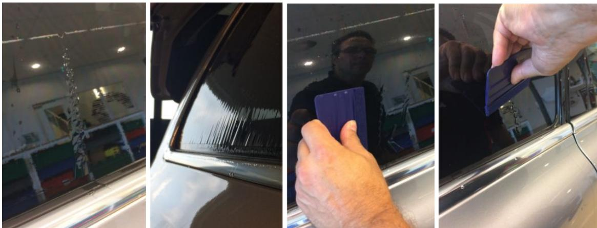
For fixed windows, after shrinking the film, cut the film to the exact side of the window, trimming the excess edges. In order not to cut directly on the car window, it is recommended to use a permanent marker to define the contour of the window on the film and then cut the film to shape. In case of roll down windows, carefully open the windows for a few centimeters. Then align the film with the top of the window and cut away any excess and also trim the corners of the film.
