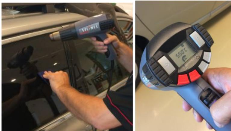
When heating, small tunnels/channels will appear on the surface. Gently squeegee them out of the film, starting from the center going towards the edges. In case large tunnels are formed, separate them in smaller tunnels using the squeegee and then remove them, following the same procedure. Ensure to shrink the whole surface of the film, carefully removing all the tunnels that are formed as explained.
