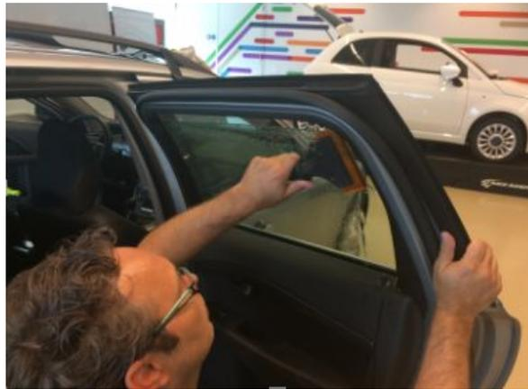
Position the film on the inside of the window and align at the top end. Make sure that the interior glass and adhesive side are sufficiently wet to allow slideability and easy positioning of the film. Be careful during this phase to avoid the formation of wrinkles on the film surface.
