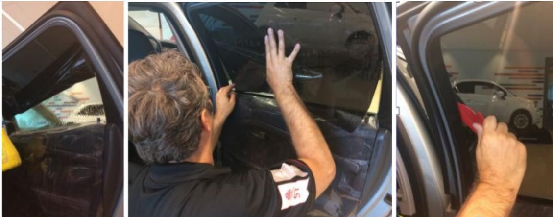
When the film is in position, re-wet the face of the film and apply uniform pressure with the squeegee to activate the adhesive and fix the film, removing all the excess water on the adhesive side.
