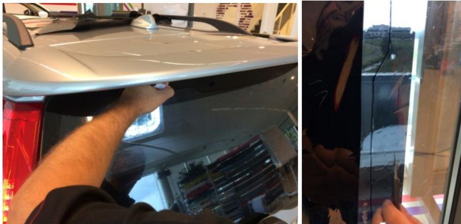
Next, prepare the inside of the rear window by cleaning and wetting it with water & soap solution to allow the film to be positioned. When wetting the interior glass, make sure to protect the interior of the car.
