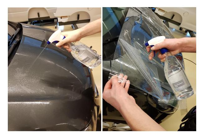
Remove the liner and spray the exposed adhesive side with the soap solution. Then position the material on the selected application area. If necessary, slide the film until you have reached the correct positioning. Pull the film to fit it to the application surface, laying it flat and removing all the wrinkles.
