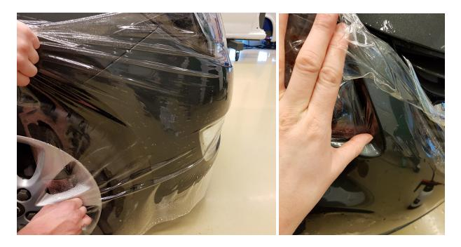
Avery Dennison Pure Defense PU presents a good degree of conformability, thus conventional convex and compound shapes on car fronts are mostly suitable to be covered with this film. Nevertheless, in deep corrugated shapes, it may be necessary to make an incision in order to avoid any form of air/water entrapment in the deep recesses. This incision does not jeopardize the functionality or durability of Avery Dennison Pure Defense PU.
