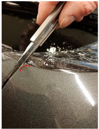
To facilitate cutting, make sure to use a new and very sharp knives for cutting: dull knives will result in blurred cutting edges. When applying Avery Dennison Pure Defense PU and PVC, it is recommended to use stainless steel blades with your knife. The use of a stainless steel blade will delay rusting and deterioration of the blades, due to contact with water.
