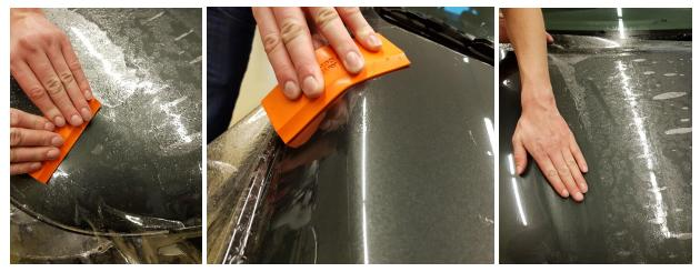
When using Avery Dennison Pure Defense PU and PVC, re-positioning of the film is only possible in the stage of initial positioning and low or no squeegee pressure. If done in a later stage small marks or lines might remain visible in the film surfaces.
