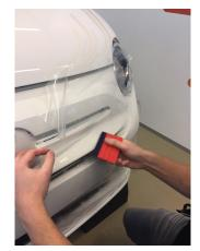
For curved areas, it is necessary to firmly pull and stretch the film in order to conform the film around the surfaces. Identifying some fixing points, where the adhesive can be activated by applying pressure, will help in the stretching and fitting process. It is recommended to stretch the material without applying any heat, making use of the intrinsic flexibility of the film. It is also possible to gently heat the material to a temperature of 40-50 °C using a heat gun or a steamer.
