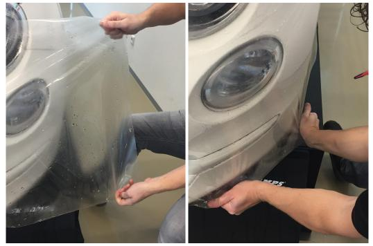
Conventional convex and compound shapes on car fronts are mostly suitable to be covered with all of the paint protection films in the Avery Dennison SPF series, but in some deeper corrugated shapes it may be necessary to make an incision in order to avoid any form of air/water entrapment in the deep recesses. This incision does not jeopardize the functionality or durability of the product.
