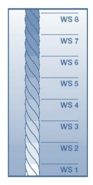
The light fastness of film inks formulated to "Euro Scale" shades is between WS 5 and WS 8. Some manufacturers offer extremely light-fast alternatives with WS values that are not below 7 or 8. The WS values can be expressed in terms of weeks and months:
