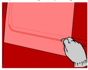
When all the deepest parts of the corrugation have been applied, the inside of the corrugation can be done. Again, make sure the material is heated to the required 40°-50°C, and work your way through the corrugation.
