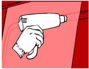
Start stretching the material in the corrugation, starting in the deepest part of the corrugation first. Make sure that the material is heated to remain in the 40°-50°C temperature range.
