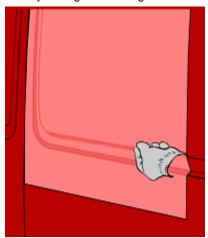
With all the edges now properly applied, apply the material in the centre of the corrugation. Make sure that no air is trapped, by always leaving an opening for the air to escape.
