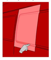
Check the application for remaining bubbles. If you see any small air bubbles, remove them by making a small puncture, heat it a little and push out the air.
