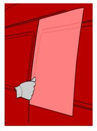
Now, the application of the material in the corrugation can start. In order to be able to do so without forming pleats or creases, it is advised to wet the glove, using a water/soap mixture.
