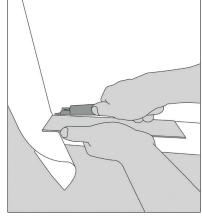
Place the squeegee next to the window silicon joint, with the cutter on the inside. Carefully cut to remove the excess, with a regular movement using strong pressure and a sharp angle. Use a new blade every 2 meters and for every corner, in order to avoid tearing the yarn.
