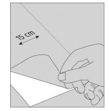
Pull out the backing paper behind Squid $^{\circ}$  on ± 15 cm and fold it.
