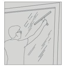
Clean and degrease the window thoroughly with water and a dash of ammoniac or alcohol. Dry the window thoroughly with a lint-free cloth.
