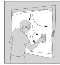
When Squid<sup>®</sup> is perfectly flat on the window, use the squeegee to adhere it well to the glass. Press from the center outwards (see arrows). Press over the entire surface well, including the edges and the corners.
