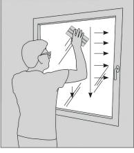
Apply a strong pressure (10 kg) with the squeegee over the whole Squid<sup>®</sup> surface, horizontally and vertically, in order to activate the glue. This is very important to avoid the formation of bubbles in Squid<sup>®</sup>.
