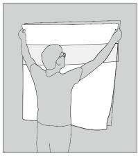
Align the Squid<sup>®</sup> with the top of the window and press the textile gently onto the glass. Take out the remaining backing paper little by little, by section of ± 15 cm each, while pressing gently the fabric onto the window from top to bottom and from the middle to the side.
