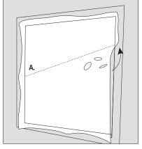
In case of bubble or crease, detach gently the fabric from the window, without applying tension, up to the level beyond the bubble or crease (A).
