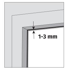
For best results, it is recommended to leave a 1-3 mm gap between the silicon joint and Squid<sup>®</sup>.
