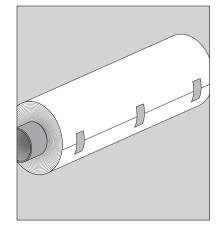
After cutting a piece of Squid<sup>®</sup>, always make sure to wrap the remaining Squid<sup>®</sup> tightly around its carton core and fix it firmly with 3 adhesive tapes evenly spread over the width of the roll. If Squid<sup>®</sup> is not kept tightly enough around the core, this might create permanent bubbles or creases in the fabric.
