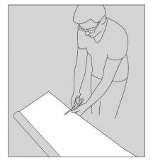
Cut the Squid<sup>\*</sup> somewhat larger than the window, adding ± 5 cm extra on each side for trimming.
