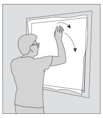
Then let it fall again smoothly onto the window, while accompanying it with your hand or with the squeegee. Never try to push out bubbles or creases by pressing with the squeegee because this would cause permanent deformations in the fabric.
