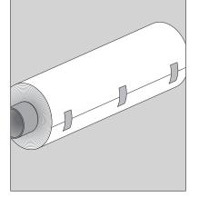
Keep Squid<sup>®</sup> tightly wrapped around its carton core until the moment of installation. It must be firmly attached with 3 adhesive tapes evenly spread over the width of the roll, in the center, left end and right end.
