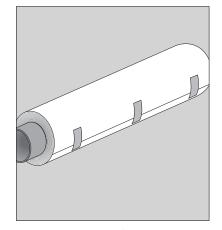
If you have some Squid<sup>®</sup> left over, keep it in its original packaging, tightly wrapped around its carton core, and firmly fixed with 3 adhesive tapes evenly spread over the width of the roll, that is in the center, left end and right end.
